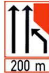
Traffic lane ends in 200m due to obstruction
