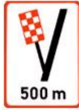
Arrester bed advance exit
