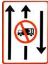
Lane control no goods vehicles in excess of 3t
