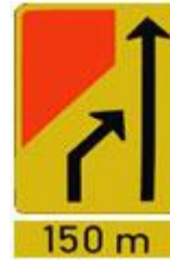
Temporary traffic movement affected by obstruction in 150m
